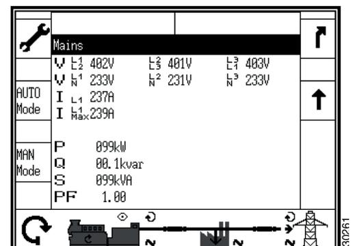
Additional measured values for the electrical power network
