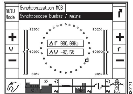
*Synchroscope busbar/electrical power network.*
