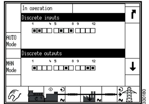
Internal digital inputs and outputs
